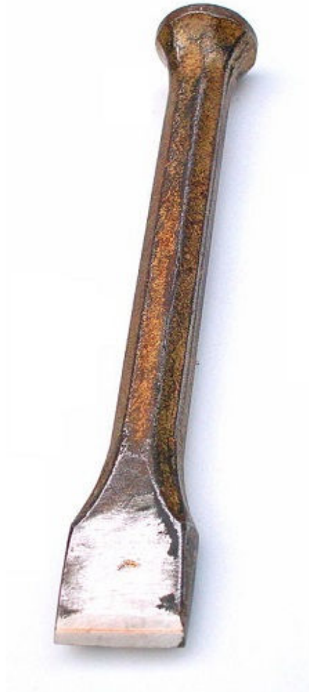
A stone chisel, with tungsten carbide carving edge, for use with a mallet. Photo: Satrughna. Source: Wikipedia.org
